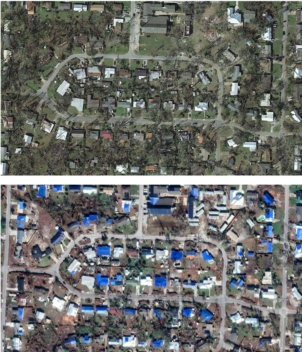
**Figure 7-3. Overhead imagery of a Panama City, FL area neighborhood in October 2018, one month after Hurricane Michael (Top) and December 2018 (Bottom). This figure shows that an example where many homes with asphalt shingle roofs required blue tarps while homes with metal roof panels did not require blue tarps as frequently.**
